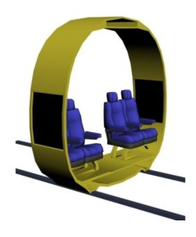
Fig. 1 – Anel do MagLev-Cobra com bancos no sentido transversal
