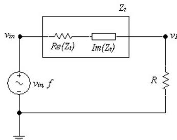
Figura 1 Schematic diagram of the circuit used to determine the impedance of a device  $Z_t$ .
