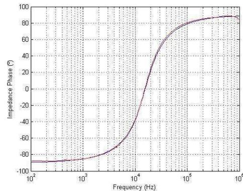
Figure 4 Phase versus frequency of a RLC serial circuit composed of a capacitance of 100 nF, an inductance of 1 mH and a resistor of 100 $\Omega$  between 100 Hz and 1 kHz (HP4294A – blue line; our system - red line).
