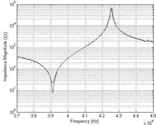
Figura 5 . Impedance versus frequency of the piezoelectric transducer between 37 kHz and 45 kHz (HP4294A - blue line; our system - red line).
