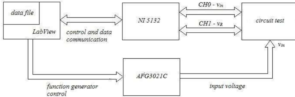
Figure 2 Block diagram of the automatic system to the determination of impedances
