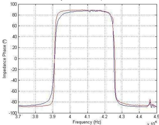
Figura 6 Phase versus frequency of the piezoelectric transducer between 37 kHz and 45 kHz (HP4294A - blue line; our system - red line).
