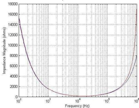
Figure 3 Impedance versus frequency of a RLC serial circuit composed of a capacitance of 100 nF, an inductance of 1 mH and a resistor of 100 $\Omega$  between 100 Hz and 1 kHz (HP4294A – blue line; our system - red line).
